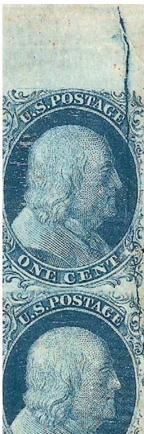
Detail of two “Big Crack” positions (2/12L) at the top of the left pane of Plate 2. The crack starts at the edge of the plate and extends down to Position 23L and, as it grew, 33L.
